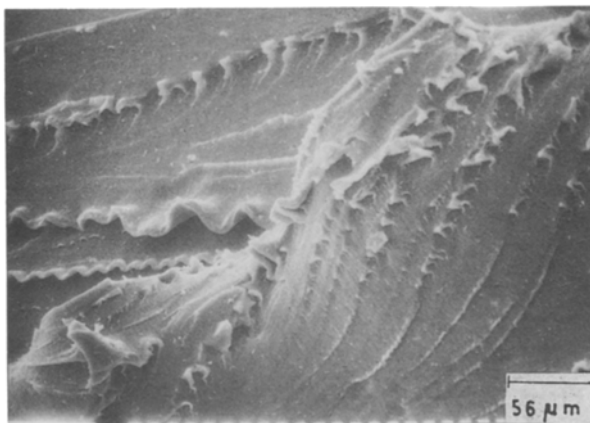
Figure 10 SEM of the tear fracture surface of PP 70 .
